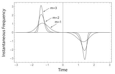
frequency because the slope of the edges of the pulses shown in the previous figure is greater for larger m.
