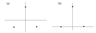
(a) Determine the mean symbol energy E in terms of d when each of the three signal points is equidistant from the origin as part (a) of the figure. Repeat for part (b). In this case, the three signal points do not have the same energy.
