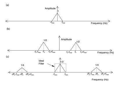
(b) Sketch the frequency spectrum  $\widetilde{S}(f)$  of the amplitude-modulated passband signal.
