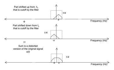
When the offset x is equal to  $f_{\text{max}}$ , the baseband spectrum is "inverted". The distortion is caused by the combination of the two parts of the spectrum not being aligned because of the different demodulation frequencies, and the lowpass filter which removes higher frequency components of the baseband signal.
