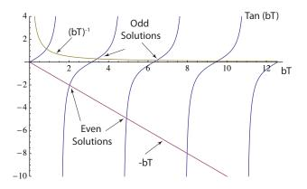
Once the values  $b_k$  are determined, the corresponding eigenvalues are given by (19) with  $b \rightarrow b_k$ . A plot of the eigenvalues for several values of  $\alpha T$  are shown in the figure below.
