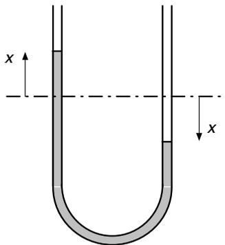
Let fluid have density  $\rho$ , tube cross-sectional area  $A$ . With a displacement  $x$  from the equilibrium position, the weight of out-of-balance fluid is
