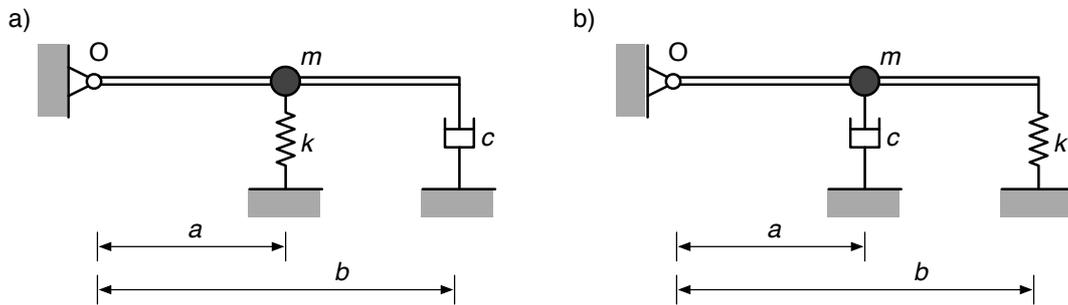
5. A damped SDOF system has mass 50 kg and stiffness 6000 N/m. When set in motion, its displacement amplitude reduces from 30 mm to 27.5 mm in one cycle. Find the damping ratio  $\xi$  and dashpot coefficient  $c$ .
