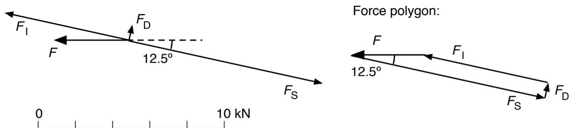
(Note on directions of vectors: the three internal force vectors must sum to give a resultant force vector equal and opposite to the applied external force  $F$ . With  $F$  assumed acting to the left, the vector sum of the three internal forces therefore acts to the right. The displacement of the mass is at a phase angle of  $12.5^\circ$  to  $F$ , and the stiffness force opposes this displacement, therefore it makes a phase angle of  $12.5^\circ$  to  $-F$ .)
