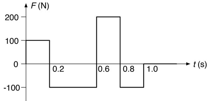
Duhamel's integral for a constant load  $F$ , undamped system, Eq 2.52:
