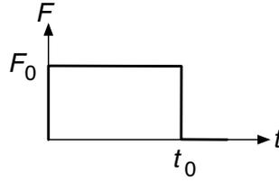
$$\bar{F}(s) = \int_0^{\infty} F(t)e^{-st} dt = \int_0^{t_0} F_0 e^{-st} dt = \left[ -\frac{F_0}{s} e^{-st} \right]_0^{t_0} = \frac{F_0}{s} (1 - e^{-st_0})$$
