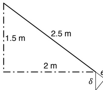
Movement consists of a cable extension  $e$ , and a perpendicular rotation. By similar triangles,  $e = 0.6\delta$ . The force in the cable is  $T = k_A e = 0.6k_A\delta$  and the vertical component of this force is  $F = 0.6T = 0.36k_A\delta$ . Therefore the vertical stiffness is:
