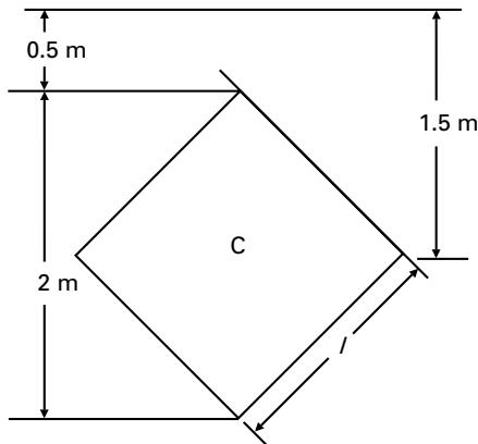
$$\begin{aligned} \text{Force on plate} \\ &= 1150 \text{ kg} \cdot \text{m}^{-3} \\ &\times 9.81 \text{ N} \cdot \text{kg}^{-1} \\ &\times 1.5 \text{ m} (\sqrt{2} \text{ m})^2 \\ &= 33.84 \text{ kN} \end{aligned}$$
