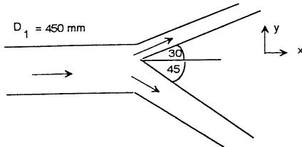
$$\begin{aligned} \text{Find } V_2, V_3 \text{ from continuity} \\ \text{Find } P_2, P_3 \text{ from Bernoulli} \\ D_3 = 300 \text{mm} \\ Q_3 = 0.34 \text{m}^3/\text{s} \\ V_3 = 4.81 \text{m/s} \\ A_3 = 0.071 \text{m}^2 \\ P_3 = 63.8 \text{kN/m}^2 \end{aligned}$$
