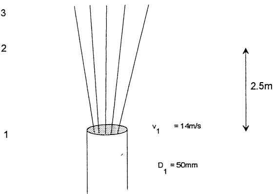
Assume atmospheric pressure at all heights and apply the energy equation.
