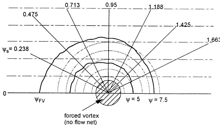
$$\text{For forced vortex } V = \omega r = 100 \times 0.15 = 15 \text{ m/s}$$
