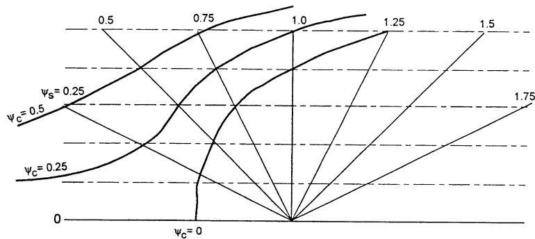
Velocity  $\rightarrow 0$  at stagnation point where radial velocity  $V_r$  is equal and opposite to velocity of linear flow i.e.  $V_r = 5 \text{ m/s}$ .
