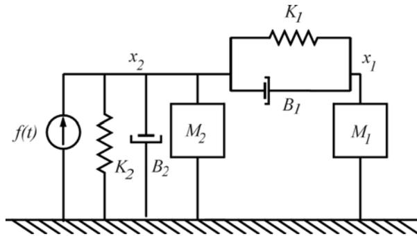
(b)  $(M_1 D^2 + B_1 D + K_1)x_1 - (B_1 D + K_1)x_2 = 0$
