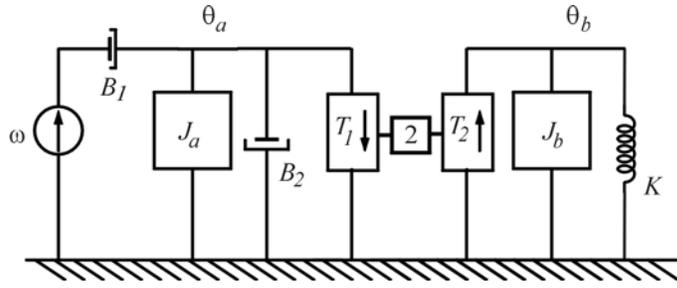
(b)  $T_1 = -(J_a D^2 + B_2 D)\theta_a + B_1 \omega$        $T_2 = 2T_1 = (J_b D^2 + K)\theta_b$
