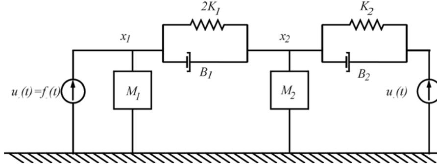
(b)  $(M_1 D^2 + B_1 D + 2K_1)x_1 - (B_1 D + 2K_1)x_2 = u_1$
