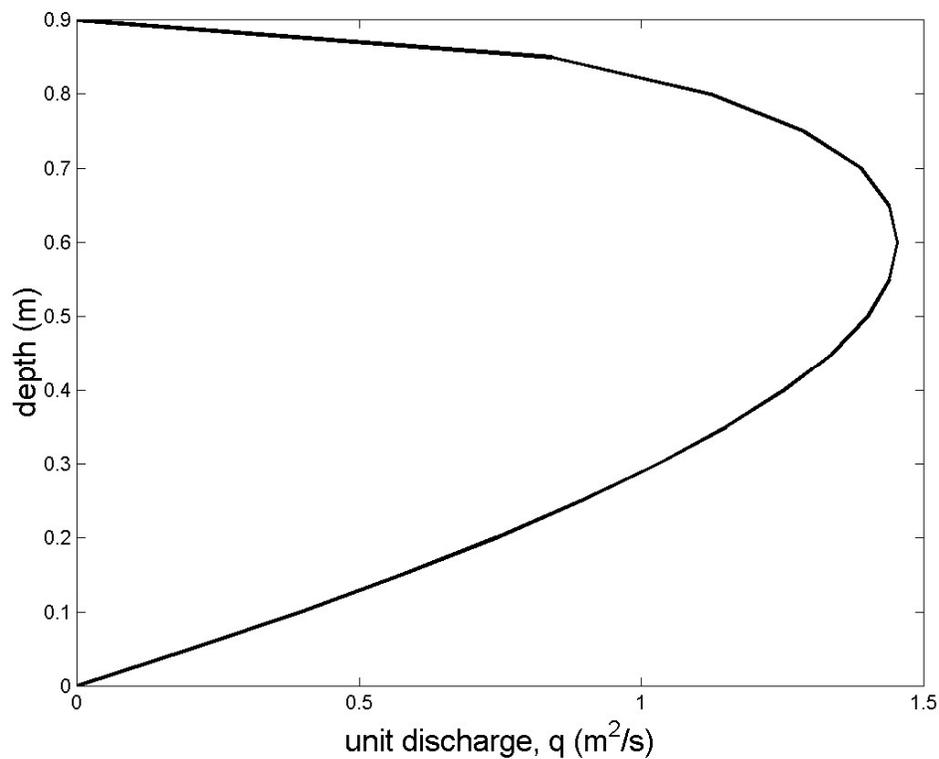
Visually, it should be clear that the unit discharge,  $q$ , is maximized at 0.6 m. This is 2/3rds of the energy provided,  $E^* = 0.9$  m
