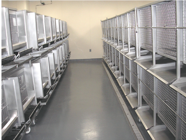
Figure 9.2 An avian toxicity testing facility in which a series of doses are fed to subsets of mallard ducks so that lethal or nonlethal effects can be quantified.
