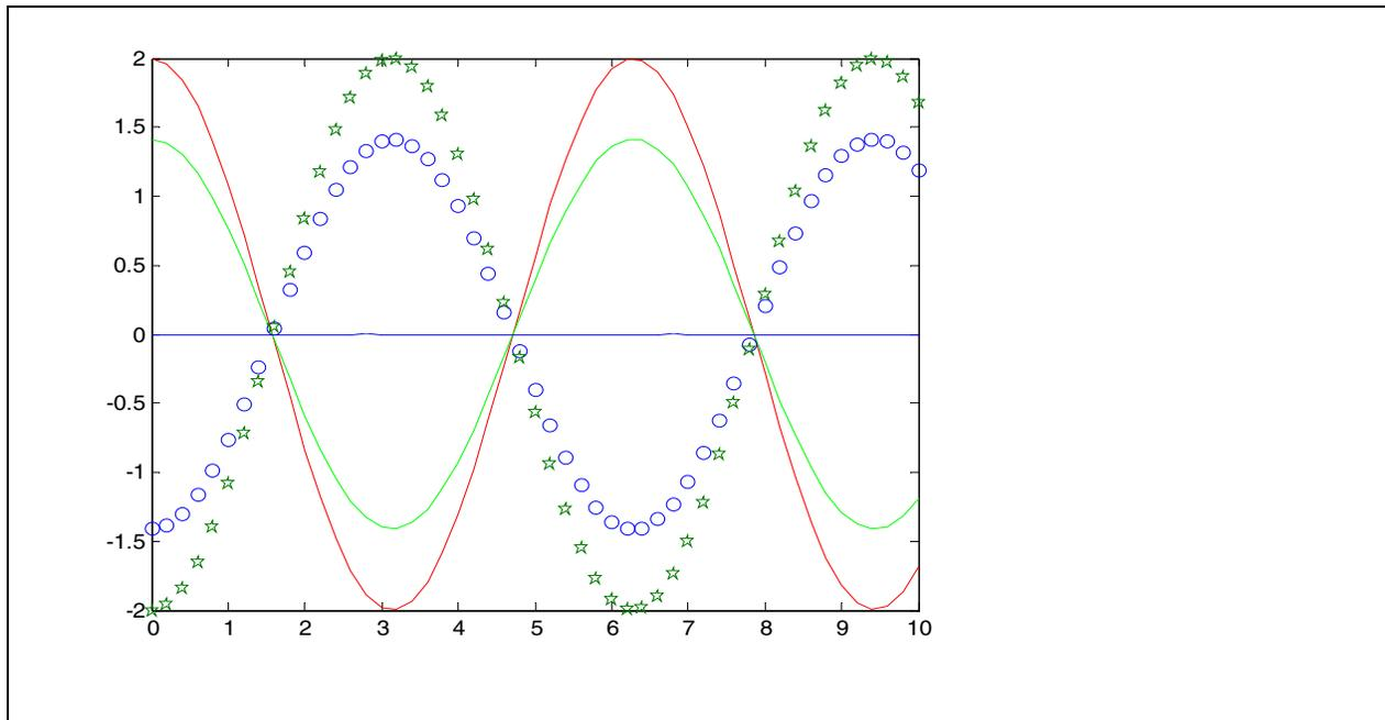
**Q-2.25** The real component of a wave traveling in a lossy media in x-direction is expressed by the following relations  $\text{Re}[E_y(x, t)] = C_1 e^{-\alpha x} \cos(\omega t - \beta x)$ . Plots  $E_y$  for  $\omega t = 0, \pi/4, \pi/2, 3\pi/4$  and  $\pi$  if  $C_1 = 1, \alpha = 1.885 \times 10^{-3}$  Nep./m and  $\beta = 0.001$  rad./m. Take  $x = 0, 0.1, 0.2, \dots, 1$
