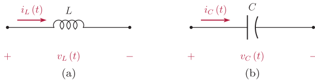
Figure 2.8 Mathematical models for (a) ideal inductor, (b) ideal capacitor.
