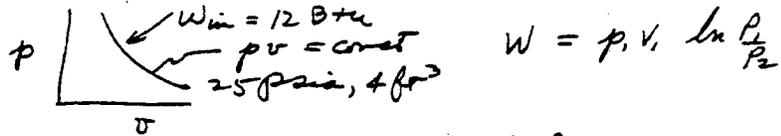
$$-12 \text{ Btu} \times 778 \frac{\text{ft} \cdot \text{lb}}{\text{Btu}} = 25 \text{ psi} \times 144 \frac{\text{in}^2}{\text{ft}^2} \times 4 \text{ ft}^3 \ln \frac{p_1}{p_2}$$
