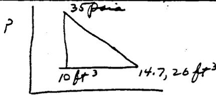
$$\text{Work} = \text{net area} = \frac{(26 - 10)(35 - 14.7) \times 144 \frac{\text{in}^2}{\text{ft}^2}}{2} = 23,385.6 \text{ ft} \cdot \text{lb}$$
