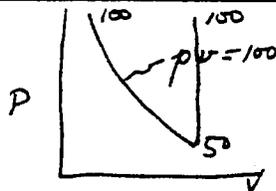
$$\text{Work} = \text{Area Under P-V Curve}$$
