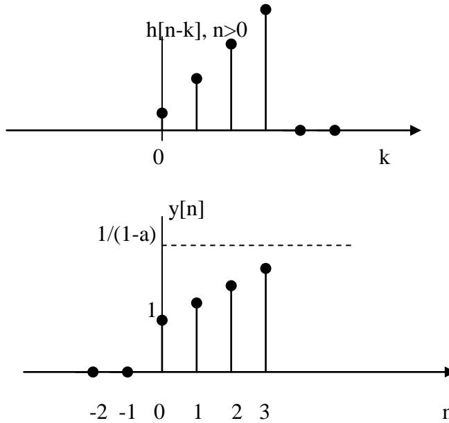
For  $n < 0$ ,  $x[k]$  and  $h[n-k]$  do not overlap. For  $n \geq 0$ , they overlap from  $k=0$  to  $k=n$ .
