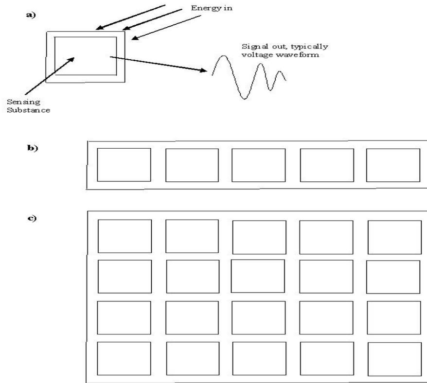
a) Single imaging sensor ; b) Linear ( line) sensor ; c) 2-D or array sensor
