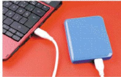
12. Storage devices like the hard disk shown in the accompanying figure often function as a source of input because they transfer items from storage to memory.
